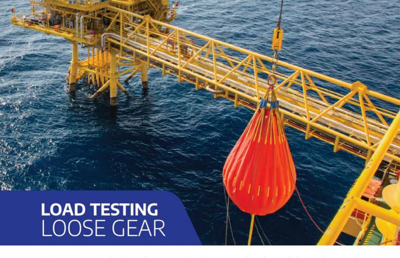
Lifting equipment can be subjected to operational and environmental conditions which may affect its safe working characteristics. Therefore, it requires that lifting equipment is properly maintained and safe to operate at all times. To ensure that, it requires pre-use inspections and interim inspections at suitable intervals by a Competent Person followed by load testing. Amar marine enterprises is capable of carrying out dynamic - static load tests for,
